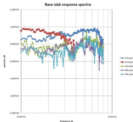
Fig. 10 – comparison of calculated vertical floor response spectra at some points in the base slab
