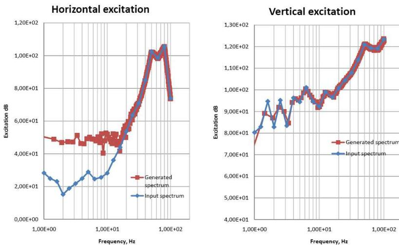
Fig. 3 – comparison of literature vibration spectra for train transit in tunnels (blue) and back-calculated spectra applied to the model (red) - a) horizontal b) vertical
