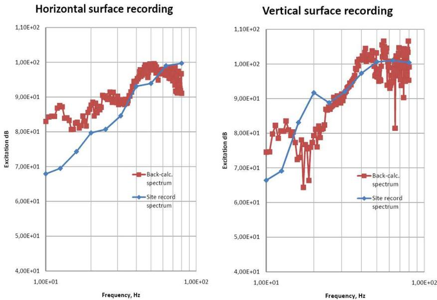
Fig. 5 – comparison of recorded vibration spectra at top of diaphragm wall (blue) and back-calculated spectra of the model (red) – a) horizontal, b) vertical
