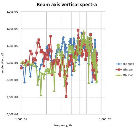
Fig. 9 – comparison of calculated vertical floor response spectra at the axis of the ground floor beams, for the 2<sup>nd</sup>, 4<sup>th</sup> and 7<sup>th</sup> span
