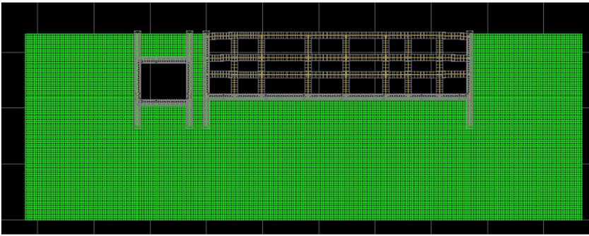
Fig. 7 – model grid, showing the tunnel and the new basement structures (grey)
