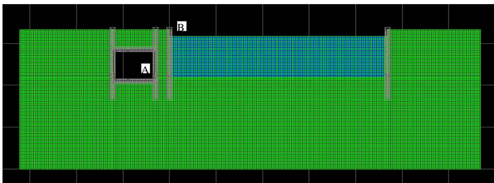
Fig. 4 – model grid, showing the tunnel structures, the new diaphragm walls (grey), future excavation soil (blue,) excitation point (A) and recording point (B)
