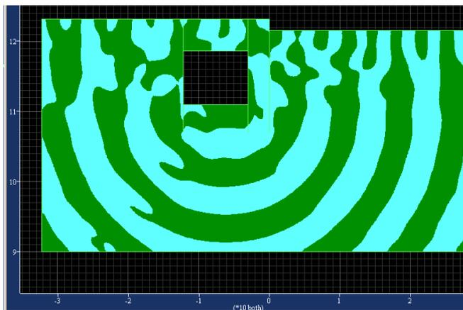
Fig. 6 – stress waves induced by a sinusoidal acceleration applied at the tunnel slab
