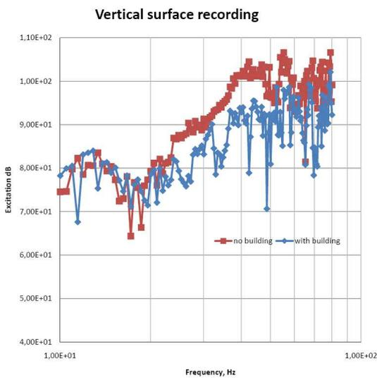
Fig. 8 – comparison of calculated spectra at top of diaphragm-wall before (red) and after (blue) the construction of the basement
