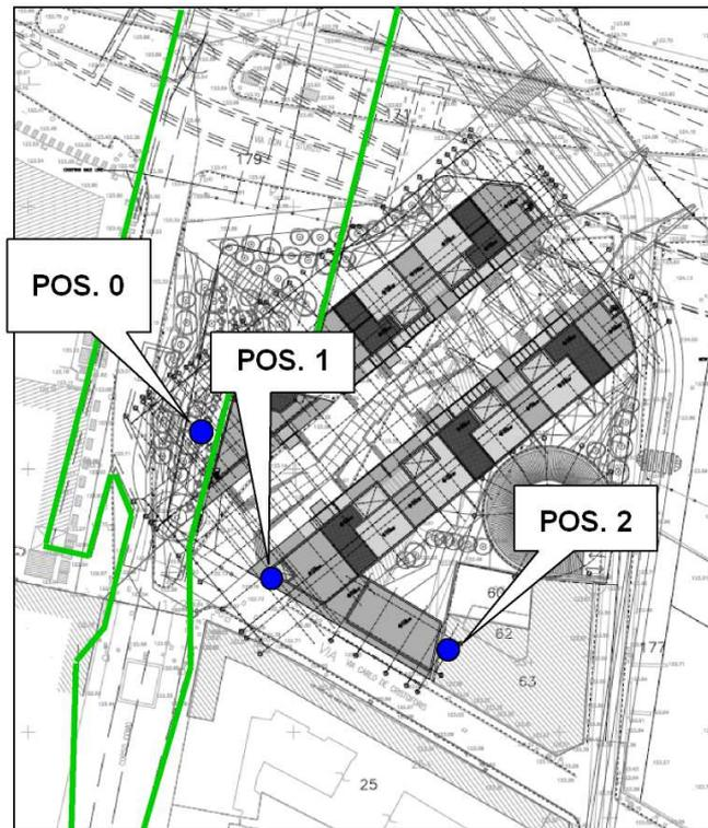
Fig. 2 – Plan view of the new buildings and of the existing tunnel (green outline)
